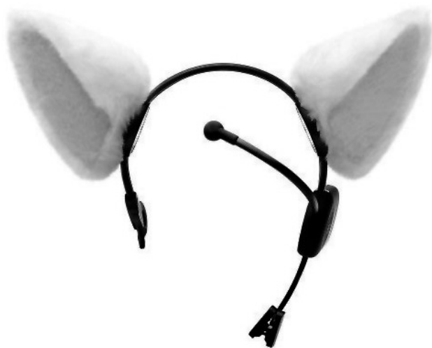
Figure 3.5 Neocomini headset with ears which move in response to electrical brain impulses
